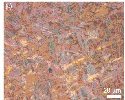
**Fig. 8** — Microstructure at surface (a), case-to-core transition zone (b), and core (c) after etching with Beraha's sulfamic acid No. 1 etch and photographing with polarized light plus sensitive tint.
