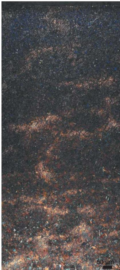
**Fig. 7** — Montage showing case-to-core transition in a carburized EX-15 alloy steel component.
