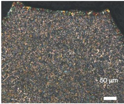
**Fig. 1** — Tooth of an 8620 alloy steel gear that failed in service. The edge of the tooth was decarburized in the heat treatment following carburizing. A 15-18  $\mu\text{m}$  deep rim along the tooth edge consists of equiaxed ferrite and pearlite. Also note that there are patches of grain boundary carbide films in a number of locations. The specimen was etched with aqueous 10% sodium metabisulfite, and the image was captured in polarized light plus sensitive tint.
