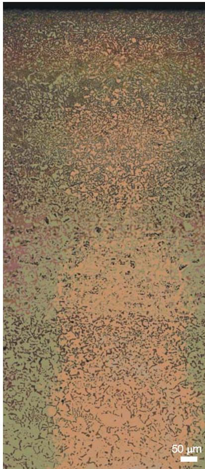
**Fig. 12 — Montage of the case-to-core transition zone on the carburized 430 stainless steel specimen etched with Murakami's reagent (20°C for 40 s) showing a region near the center relatively free of Cr<sub>7</sub>C<sub>3</sub> carbides.**
