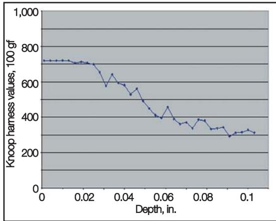
**Fig. 9** — Knoop hardness traverse for the EX-15 carburized specimen showing a relatively uniform hardness in the case to a depth of about 0.025 in.
