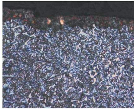
**Fig. 2** — Higher magnification views of the surface of the failed 8620 gear showing the surface with Nomarski DIC (left) and with polarized light plus sensitive tint (right). Note the decarburized pearlitic surface layer with patches of ferrite and the grain-boundary cementite networks. The matrix is coarse plate martensite with substantial retained austenite.
