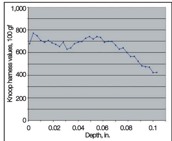
**Fig. 5** — Knoop hardness traverse of poorly carburized and heat treated 8620 specimen showing erratic hardness readings in the region to a depth of about 0.03 in. (~ 800  $\mu\text{m}$ ) due to the high amount of retained austenite and the grain boundary carbide networks in this area.
