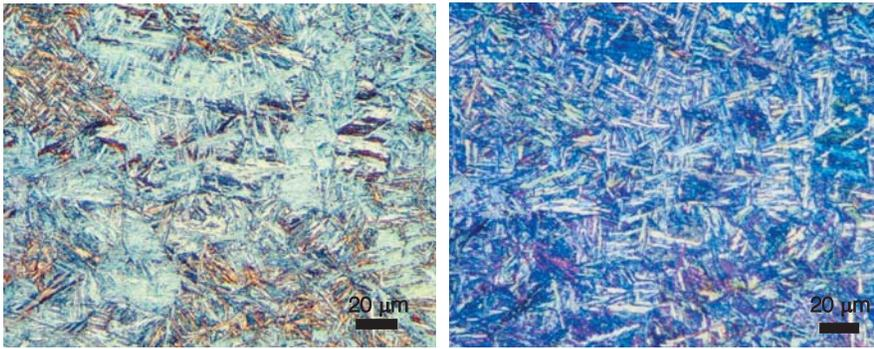
Fig. 15 — Lower bainite structure of the case revealed by etching with aqueous 10% sodium metabisulfite: bright field (left); polarized light and sensitive tint (right).
