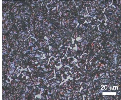
**Fig. 3** — Microstructure of the case below the surface showing the grain-boundary carbide network patches and the matrix of retained austenite and plate martensite. The image was taken using Nomarski DIC after etching with aqueous 10% sodium metabisulfite.
