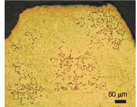
**Fig. 4** — Grain boundary carbide networks revealed by etching with alkaline sodium picrate at 90°C for 90 s. This etch will color cementite ( $\text{M}_3\text{C}$ ) and also will color  $\text{M}_7\text{C}_3$ , but that carbide type cannot form in carburized 8620.
