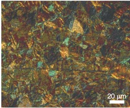
**Fig. 6** — Core microstructure consists of lath martensite and a minor amount of bainite. The specimen was etched with aqueous 10% sodium metabisulfite and was photographed with polarized light and sensitive tint.
