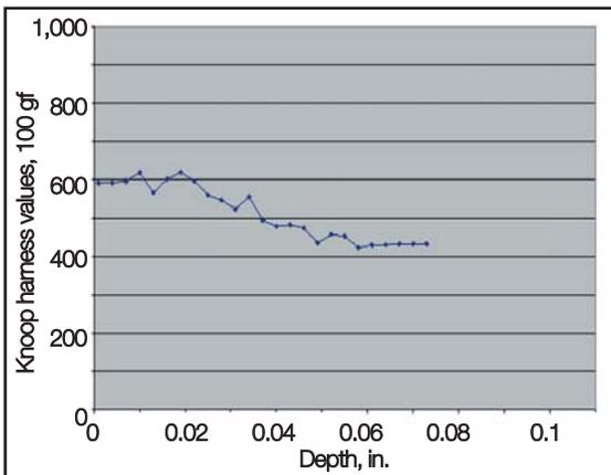
Fig. 17 — Knoop hardness traverse for carburized 8620 where the case was isothermally transformed to lower bainite and the core is lath martensite.
