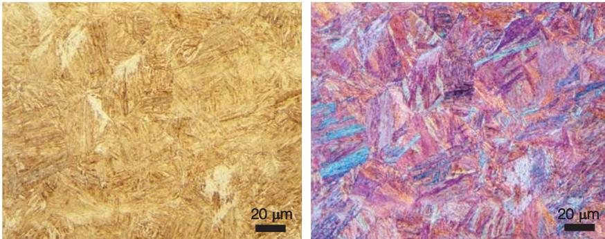
Fig. 16 — Lath martensite structure of the core revealed by etching with aqueous 10% sodium metabisulfite: bright field (left); polarized light and sensitive tint (right).
