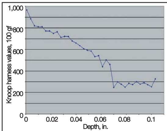
**Fig. 13 — Knoop hardness traverse for the carburized 430 ferritic stainless steel specimen. The effective case depth is ~0.058 in. (~1,485 μm, or 1.49 mm).**
