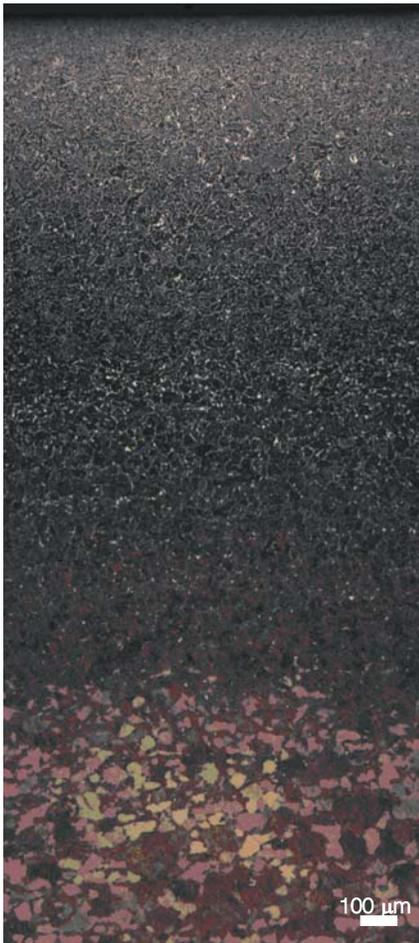
**Fig. 10 — Montage of a carburized 430 stainless steel specimen showing the case-to-core transition after etching with Beraha's sulfamic acid etch # 4 and photographing under polarized light plus sensitive tint.**
