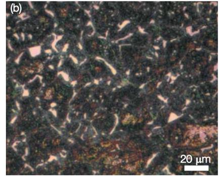
**Fig. 11 — Very heavy carbide concentration at the surface (a) and in the transition zone (b) of the carburized 430 ferritic stainless steel specimen etched with Beraha's sulfamic acid reagent No. 4. The matrix is tempered martensite.**
