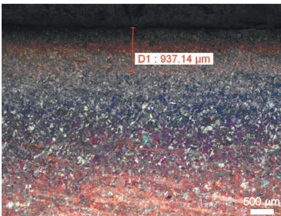
Fig. 18 — Visual estimate of the case-to-core transition depth, 937 µm (~0.0365 in.), which corresponds to a hardness of 556 HK; specimen was etched with Beraha's sulfamic acid No. 1 reagent and photographed in polarized light plus sensitive tint at 50x.
