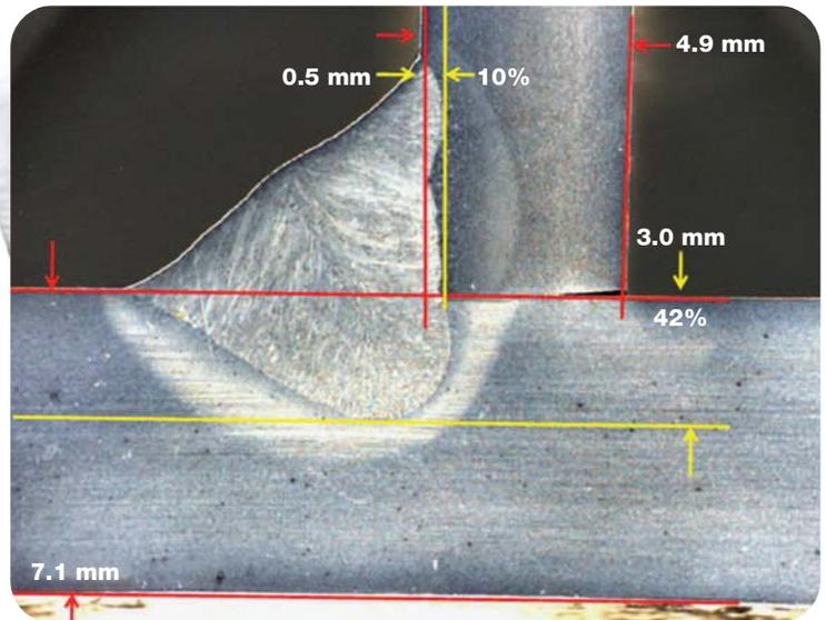
**Fig. 6** — An example of weld penetration depth measurements using the Welding Expert.
