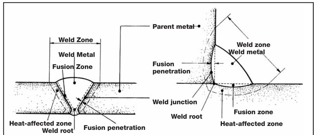
Fig. 1 — Weldment terminology for a butt weld (left) and a fillet weld (right). Source: AWS A3.0: 2001.
