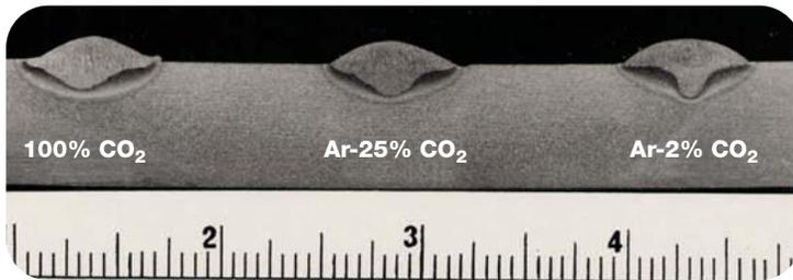
**Fig. 3** — Macrostructure of three GMA welds in a structural steel with a heat input of 45 kJ/in. and atmospheres of 100% CO<sub>2</sub>, argon plus 25% CO<sub>2</sub>, and argon plus 2% O<sub>2</sub>. Etched with aqueous 10% nitric acid.
