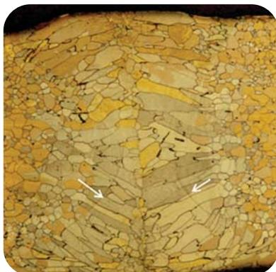
**Fig. 8** — Grain structure of a friction butt weld in Type 439 ferritic stainless steel etched using Beraha's sulfamic acid reagent (No. 4) and viewed using bright field illumination at 50 $\times$ . The arrows point to faint strain lines in the weldment.
