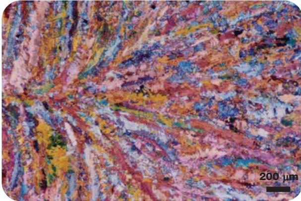
**Fig. 10** — Microstructure of a spot weld (weld only) made between two 350-MPa HSLA steel sheets revealed by Beraha's sulfamic acid reagent No. 1 and viewed using polarized light plus sensitive tint.
