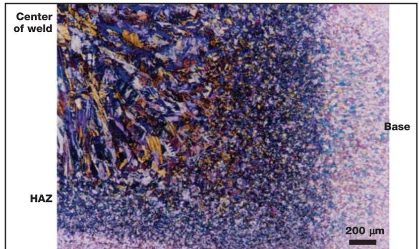
**Fig. 9** — Microstructure of a spot weld in a deep-drawing quality C-Mn sheet steel revealed using Klemm's I reagent and polarized light plus sensitive tint.
