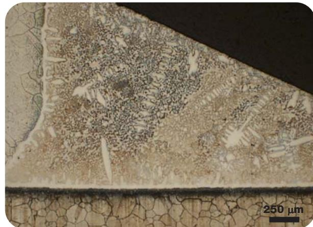
**Fig. 12** — Braze using Microbrazo LM (Ni-7Cr-3Fe-3.1B-4.5S) between K-Monel (left) and Type 304 stainless steel (below). Note carbide precipitation (sensitization) in the heat affected zones. Etch: 14 mL water, 100 mL HCl, 3 mL HNO<sub>3</sub>, and 20 g FeCl<sub>3</sub> dissolved in 20 mL water.
