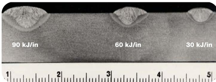
**Fig. 4** — Macrostructure of submerged arc welds in structural steel with heat inputs of 90, 60, and 30 kJ/in. (left to right); etched with aqueous 10% nitric acid.
