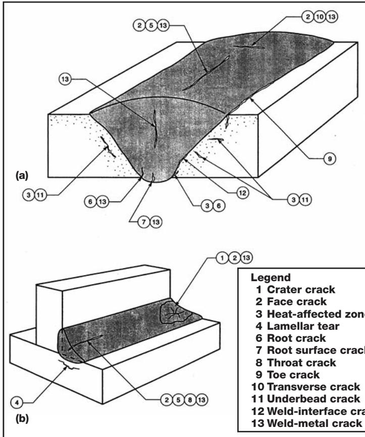
**Fig. 2** — Terminology for describing cracks in welds. Source: AWS A3.0: 2001.
