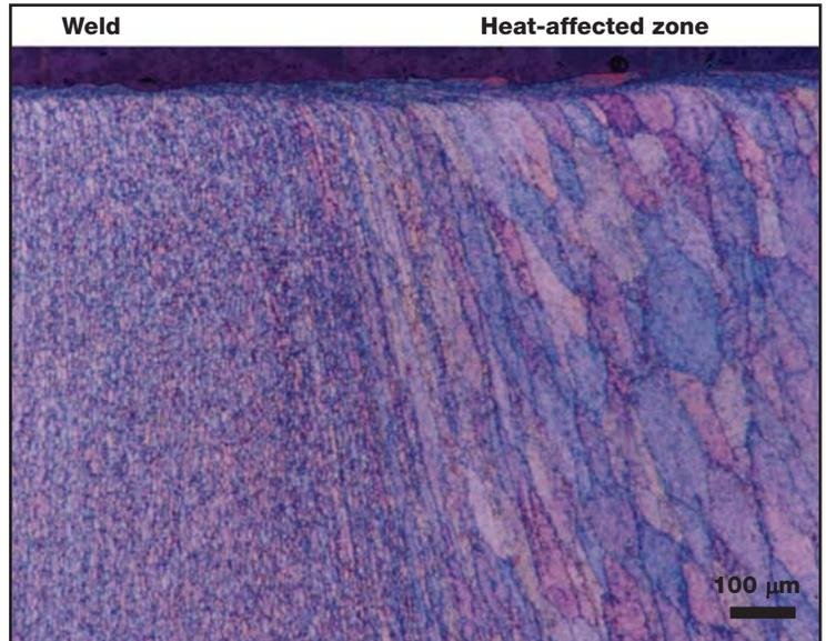
**Fig. 11** — Microstructure of a friction stir weld in 2519 aluminum alloy (Al - 5.8% Cu - 0.3% Mn - 0.3% Mg - 0.06% Ti - 0.1% V - 0.15% Zr) etched using Weck's reagent and viewed using polarized light plus sensitive tint.
