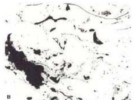
Fig. 12. Bright field views of the AMS 7875 (a) and PWA 1337 (b) coatings after etching with Murakami's reagent at room temperature. The structure of the AMS 7879 coating was heavily attacked by this reagent (although it is commonly used to etch WC-Co sintered cutting tool materials) and is not shown
