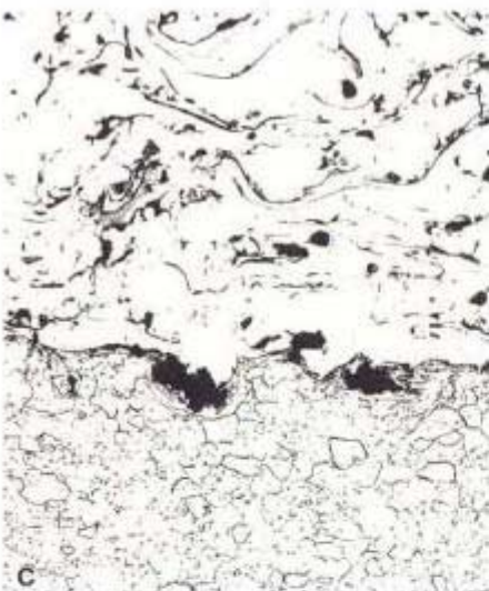
Fig. 11. Bright field, etched views of the specimens vacuum impregnated and mounted in Caldofix containing Epopdye: a) AMS 7875; b) AMS 7879; c) PWA 1337. The specimens were vibratory polished with OP-S colloidal silica for 50 minutes before etching with waterless Kallings reagent. The etchant revealed the substrate structure, but little else
