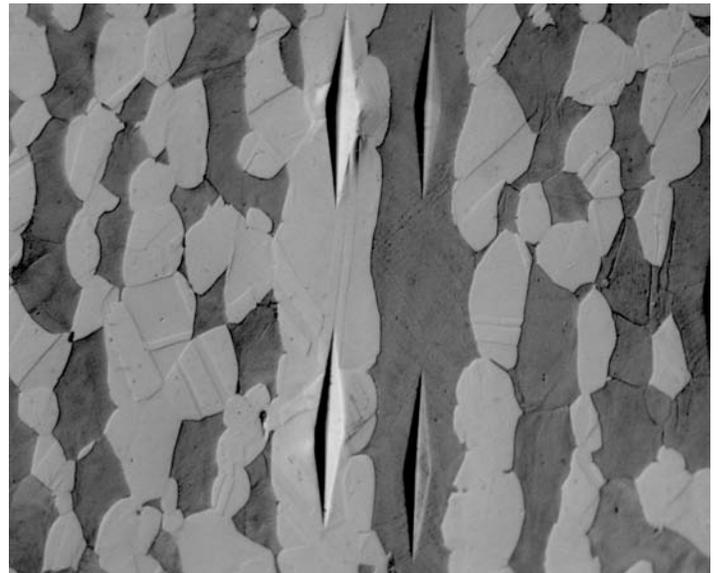
**Fig. 22** Knoop indents (50 gf) in alpha (white) and beta (dark) grains in naval brass (C 46400) (differential interference contrast illumination, Klemm's I reagent). 500x
