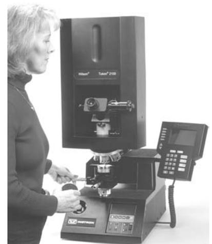
**Fig. 5** Closed-loop load-cell microindentation hardness tester
