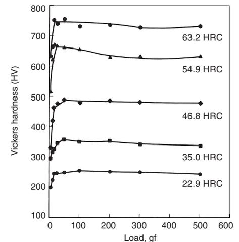
**Fig. 13** Measured Vickers microindentation hardness for five steel test blocks using test forces from 5–500 gf. Source: Ref 3
