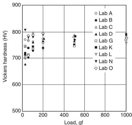
**Fig. 14** ASTM E-4 round-robin interlaboratory Vickers microindentation hardness-testing data for the hardest (F1) test specimen and nine people (measuring the same indents) who produced “good” data for test loads from 25–1000 gf. Source: Ref 6, 7
