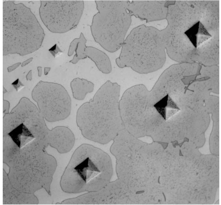
**Fig. 24** Vickers indents (50 gf) in the matrix (dark) and in the intergranular beta (white) phase in as-cast beryllium copper (C 82500) that was burnt in solution annealing (differential interference contrast illumination, aqueous 3% ammonium persulfate and 1% ammonium hydroxide). 500x
