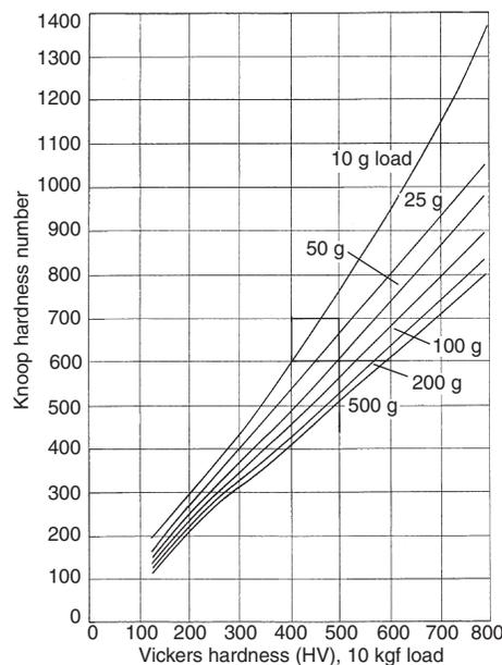
Fig. 7 Correlations between Vickers hardness determined with a 10 kgf load and Knoop hardness determined with loads from 10–500 gf. Source: Ref 1
