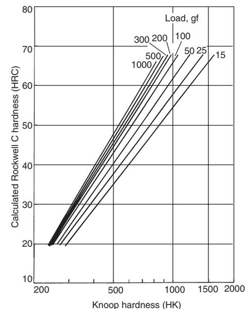
Fig. 8 Correlations between Knoop hardness at loads from 15–1000 gf and Rockwell C hardness. Source: Ref 2
