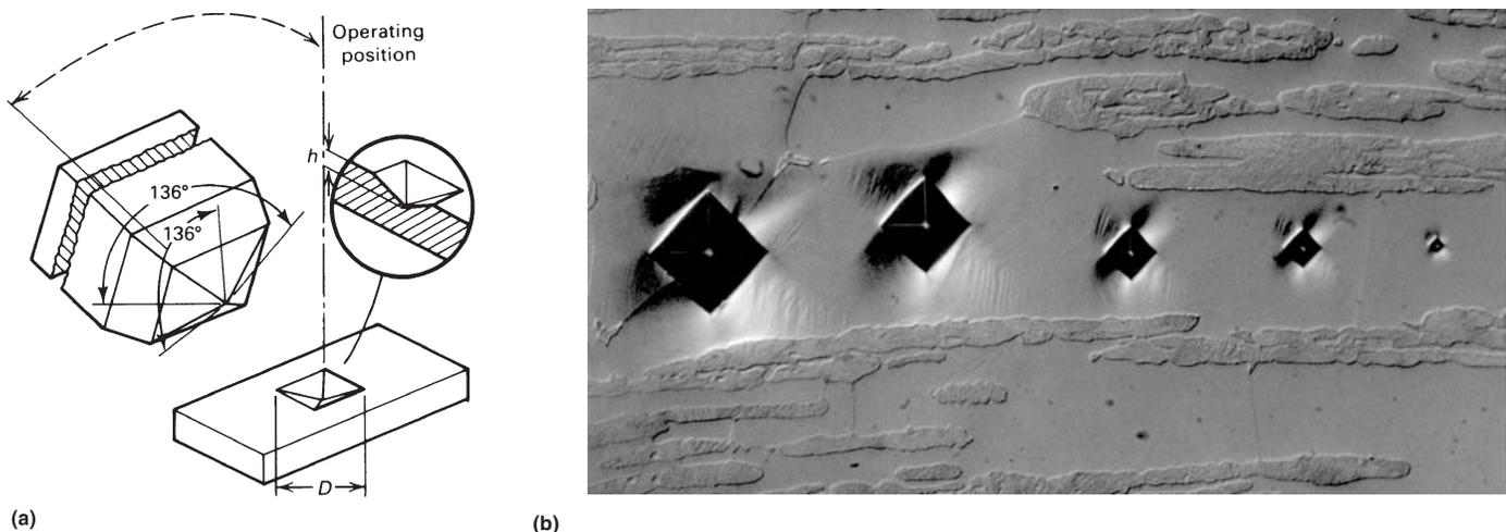
**Fig. 1** Vickers hardness test. (a) Schematic of the square-based diamond pyramidal indenter used for the Vickers test and an example of the indentation it produces. (b) Vickers indents made in ferrite in a ferritic-martensitic high-carbon version of 430 stainless steel using (left to right) 500, 300, 100, 50, and 10 gf test forces (differential interference contrast illumination, aqueous 60% nitric acid, 1.5 V dc). 250x
