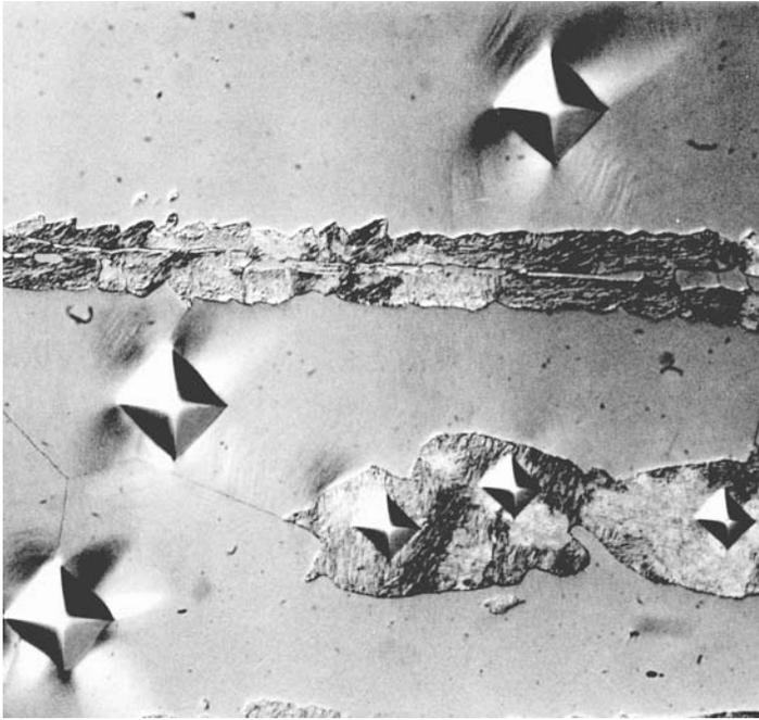
**Fig. 23** Vickers indents (100 gf) in alpha (white) and martensite (dark) grains in a high-carbon version of 430 stainless steel (differential interference contrast illumination, aqueous 60% nitric acid, 1.5 V dc). 500x
