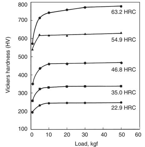
**Fig. 12** Measured Vickers macrohardness for five steel test blocks using test forces from 1–50 kgf. Source: Ref 3
