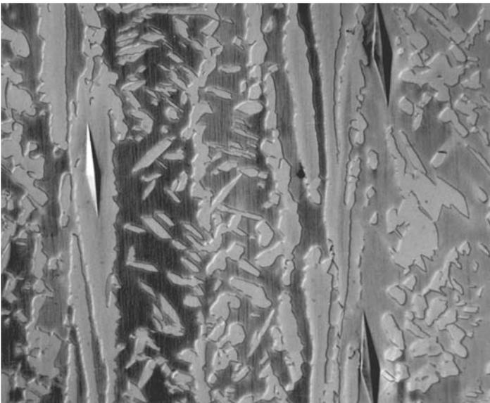
**Fig. 21** Knoop indents in ferrite (dark) and austenite (white) grains in a dual-phase stainless steel (differential interference contrast illumination, aqueous 20% nitric acid, 3 V dc). 500x
