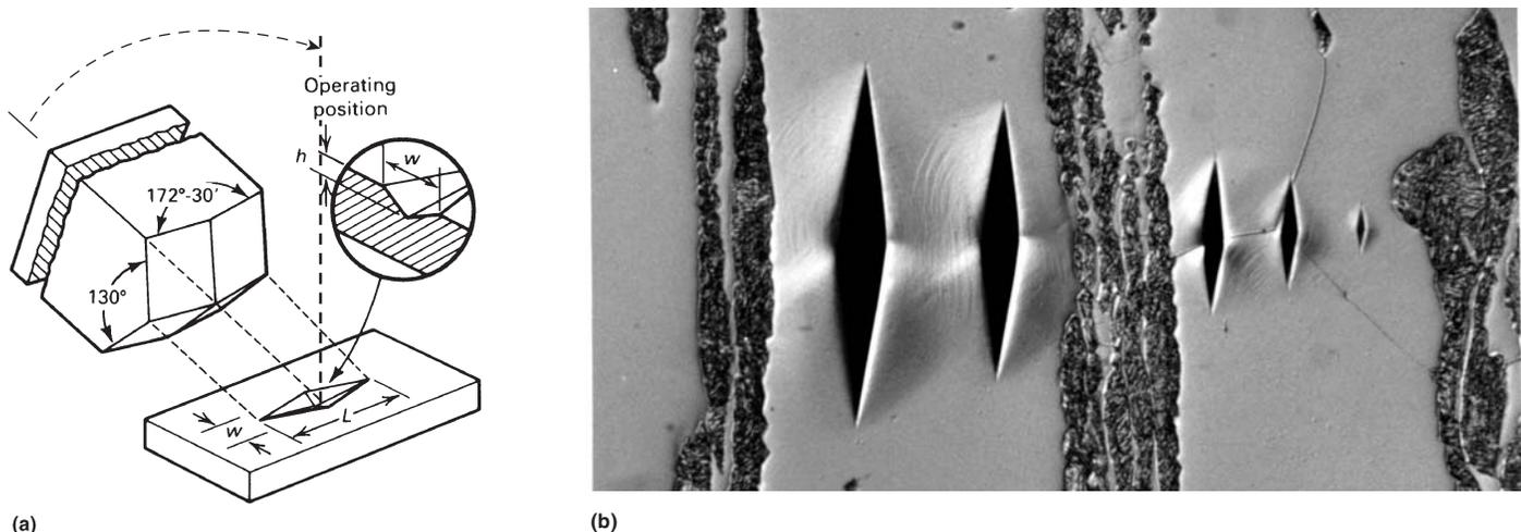
**Fig. 2** Knoop hardness test. (a) Schematic of the rhombohedral-shaped diamond indenter used for the Knoop test and an example of the indentation it produces. (b) Knoop indents made in ferrite in a ferritic-martensitic high-carbon version of 430 stainless steel using (left to right) 500, 300, 100, 50, and 10 gf test forces (differential interference contrast illumination, aqueous 60% nitric acid, 1.5 V dc). 300x
