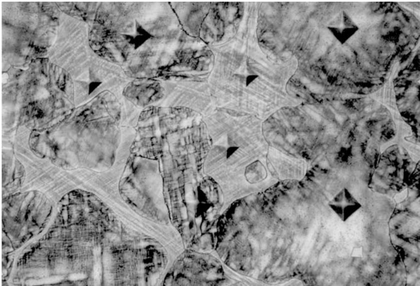
**Fig. 25** Vickers indents (100 gf) in the matrix (dark) and in the intergranular beta (white) phase in an age-hardened as-cast beryllium copper (C 82500) that was burnt in solution annealing (differential interference contrast illumination, aqueous 3% ammonium persulfate and 1% ammonium hydroxide). 500x
