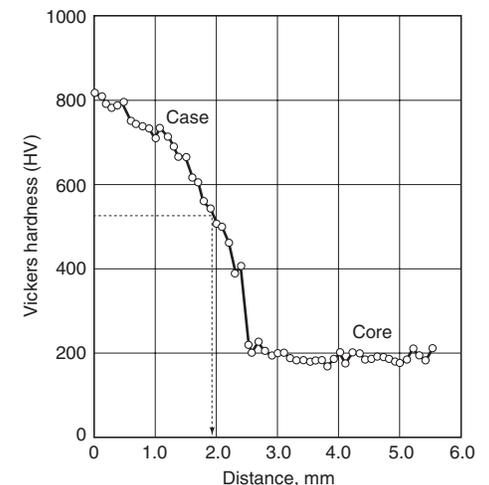
**Fig. 18** Vickers traverse showing the hardness profile results from a flame-hardened SAE 8660 gear using a fully automated microindentation hardness-testing system
