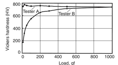
**Fig. 16** Curves showing load versus Vickers hardness for two testers (with the same operator) evaluating the hardness of the same type 440C martensitic stainless steel specimen (62.7 HRC)
