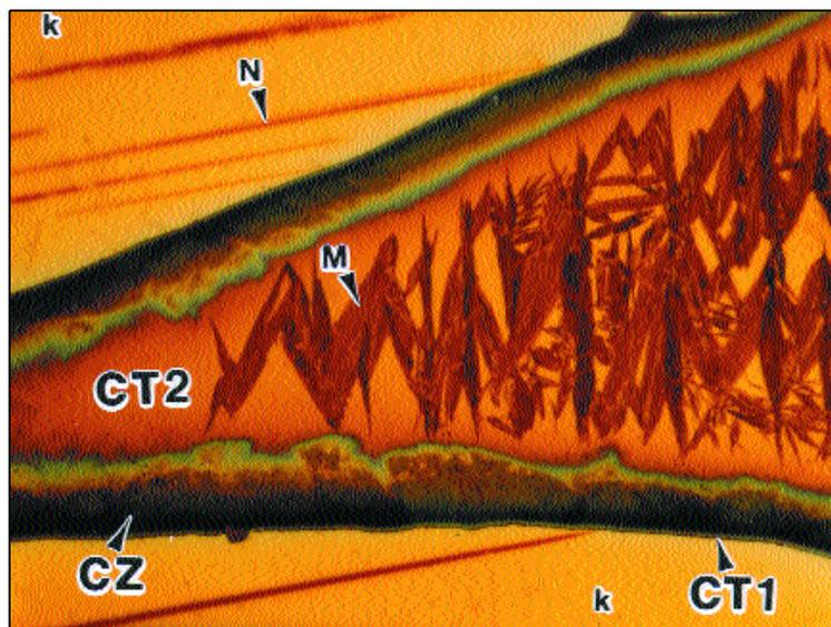
*Fig. 1 — Color micrograph (400X) of Odessa, a coarse octahedrite, etched with Beraha's complex CdS tint etch revealing a taenite wedge containing a clear taenite outer rim (CT1), a cloudy zone (CZ), an inner clear taenite zone (CT2,) and martensite (M), surrounded by kamacite (k) containing Neumann bands (N). Beraha's etch.*
