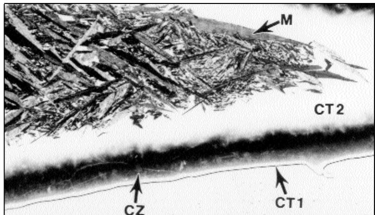
Fig. 4 — A large patch of taenite containing a thin outer layer of clear taenite (CT1), a dark etching cloudy zone (CZ), an inner region of clear taenite (CT2) and martensite (M) in the central region in the Canyon Diablo meteorite, a coarse octahedrite that fell in Arizona (etched with 2% nital, 400X).
