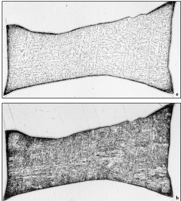
Fig. 3 — An example of finger plessite in Gibeon, a fine octahedrite that fell in Southwest Africa. (a) etched in 4% picral; (b) etched in 2% nital (200X).
