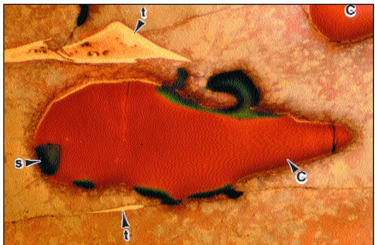
Fig. 10 — The microstructure of the Canyon Diablo meteorite. It was etched with Beraha's selenic acid tint etch.
