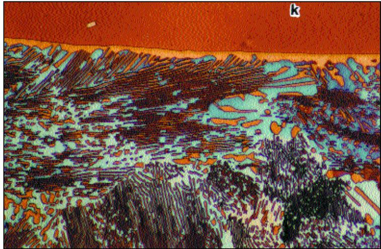
Fig. 8 — Color micrograph of Arispe, a coarse octahedrite that fell in Mexico, tint-etched with Beraha's complex CdS tint etch. It reveals (400X): kamacite (k), plessite where both the kamacite and taenite are colored, and cohenite (C).
