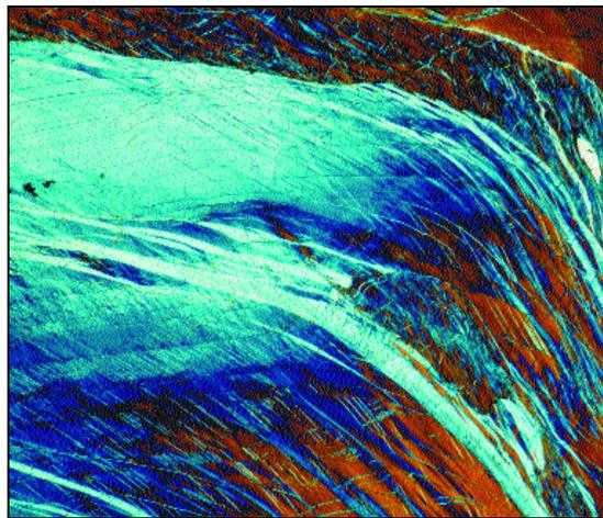
Fig. 9 — The Henbury meteorite after etching with sodium thiosulfate and potassium metabisulfite. Henbury is a medium octahedrite that fell in Australia.
