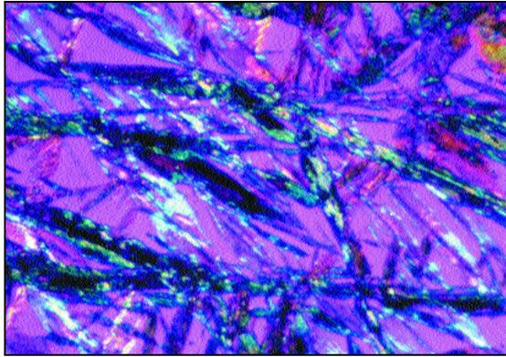
Fig. 5 — Martensite in a patch of taenite (colored magenta) in Odessa observed using nearly crossed polarized light and a sensitive tint plate (etched with 2% nital, 1000X).
