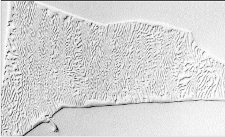
Fig. 2 — A patch of plessite, a mixture of kamacite and taenite, surrounded by kamacite in Odessa, a coarse octahedrite that fell in Texas, viewed with DIC at 400X in the as-polished condition.
