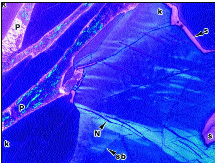
Fig. 6 — Color micrograph of Odessa, a coarse octahedrite, tint etched with sodium metabisulfite and viewed with nearly crossed polarized light and sensitive tint revealing (50X): plessite (P), Neumann bands (N), schreibersite (s), kamacite (k) and subgrain boundaries (sb).
