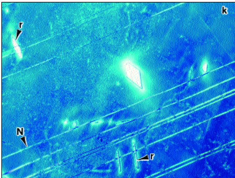
Fig. 7 — Color micrograph of Coahuila, a hexahedrite that fell in Mexico, after tint etching with sodium thiosulfate and potassium metabisulfite revealing (200X): kamacite (k), Neumann bands (N), prismatic-shaped and plate-shaped rhabdites (r).
