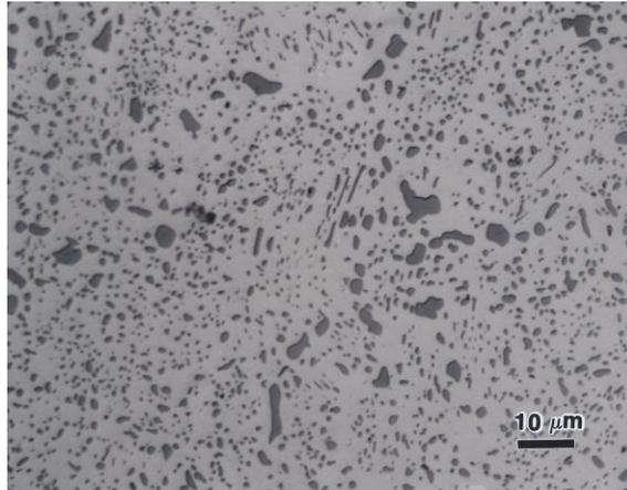
Figure 2. Spheroidize annealed W1 water-hardened carbon tool steel etched with (left) 4% picral to reveal the general structure, with (right) Klemm's I to color the ferritic matrix, and with (center, below) alkaline sodium picrate at 90 °C for 60 seconds to color the cementite.
